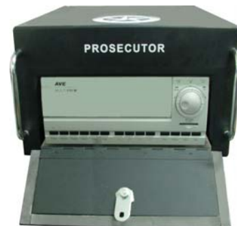
Figure 6 : DVR in Vault
