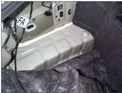
Partially remove carpet from work area.
