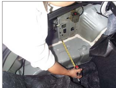
Measure 3-7/8" out from the edge, use 17/64 metal drill bit to drill a hole.
