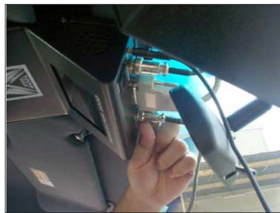
View of DB-25, interface, LED, camera and power cables being connected to control head.
