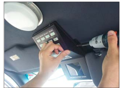
View of control head being mounted with wires already attached to connections
